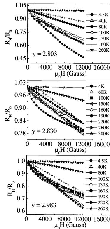
FIG. 5. Magnetoresistance for  $\text{La}_{0.5}\text{Ca}_{0.5}\text{MnO}_y$  samples showing the insulator–metal transition.
