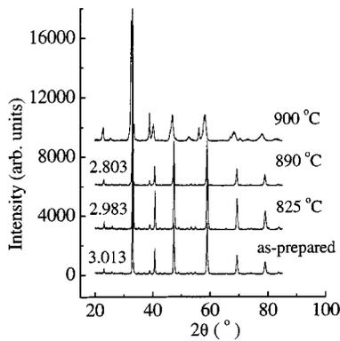
FIG. 1. X-ray diffraction patterns of the as-prepared  $\text{La}_{0.5}\text{Ca}_{0.5}\text{MnO}_y$  sample and samples annealed at different temperatures.
