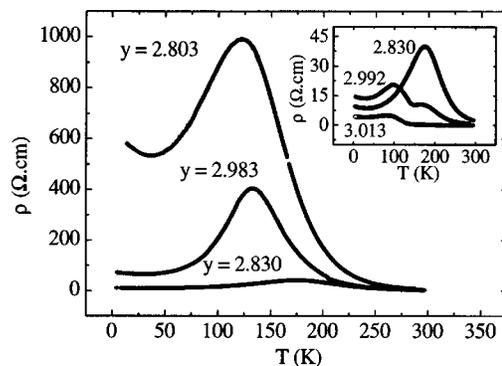
FIG. 3. Temperature dependence of resistivity for  $\text{La}_{0.5}\text{Ca}_{0.5}\text{MnO}_y$  samples with different oxygen contents.
