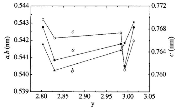
FIG. 2. Variation of the lattice parameters  $a, b, c$  with oxygen content for  $\text{La}_{0.5}\text{Ca}_{0.5}\text{MnO}_y$ .
